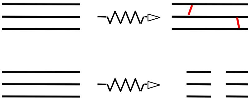
Figure 1-3. Scheme of radiation effects of polymers; cross-linking (top), degradation (bottom).
