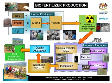
Figure 1. Flow Chart of Biofertilizer Production
