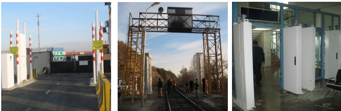
Figure 3: Gamma/neutron detection at the border ports for passenger, vehicle and rail monitoring
