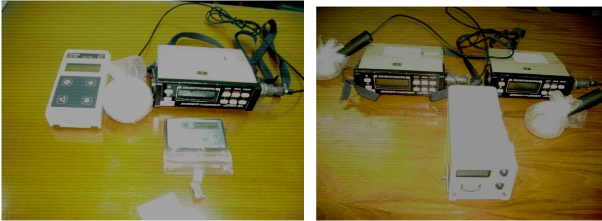
Figure 6: Radiation survey meters used for the measurement of dose rate
