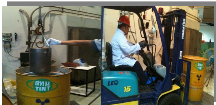
Fig 5. Activated Parts (SS) in shielded container and storage at WMC
