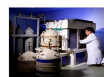
Anticoincidence-Shielded HPGe γ-Spectrometry
