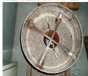
Fig 6. Drum Preparation and source immobilization in cement matrix
