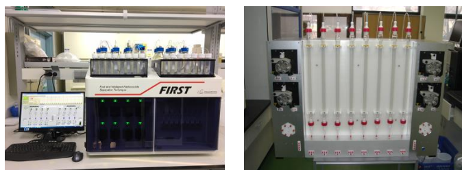
Figure 5 Automated radionuclide separation system (left: for small volume of sample, right: for large volume of sample)
