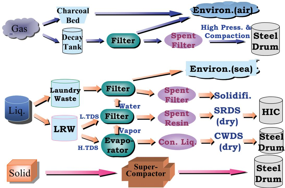
Fig. 3.5-2 Radioactive Waste Treatment Process Flow
