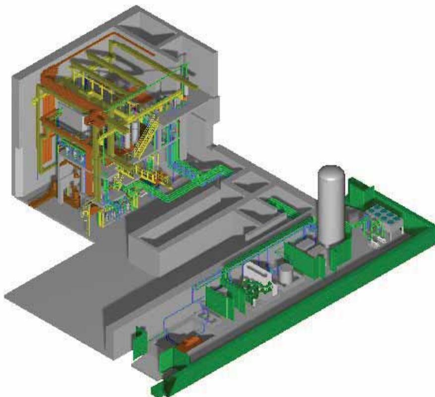
**Fig. 3.5-3 Bird's eye of Ulchin vitrification facility**
