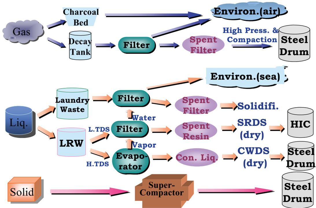
Fig. 3.5-2 Radioactive Waste Treatment Process Flow
