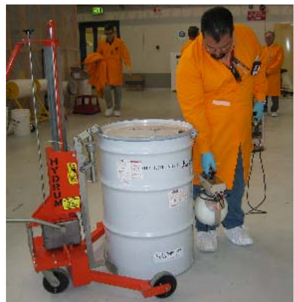
Type A Package with Pu-239/Be source
