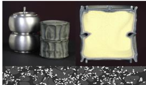
Waste immobilised in SYNROC process
