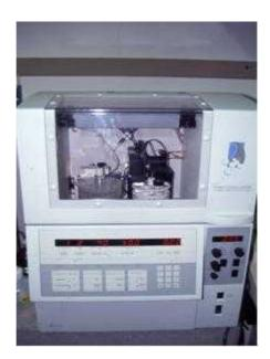
Fig. 9: Apparatus of Capillary Electrophoresis
