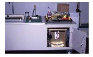
Fig. 7: Photograph of <sup>15</sup>N analyzer by emission spectrometry (JASCO Ltd N-150 analyzer)
