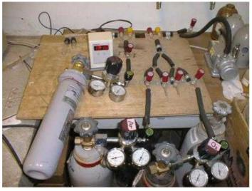
Fig 11: Gas mixing apparatus for  ${\rm ^{15}N_2}$  fixation studies
