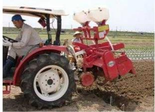
Fig.2: Fertilizer application by deep placement method
