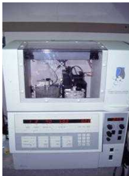
Fig. 9: Apparatus of Capillary Electrophoresis
