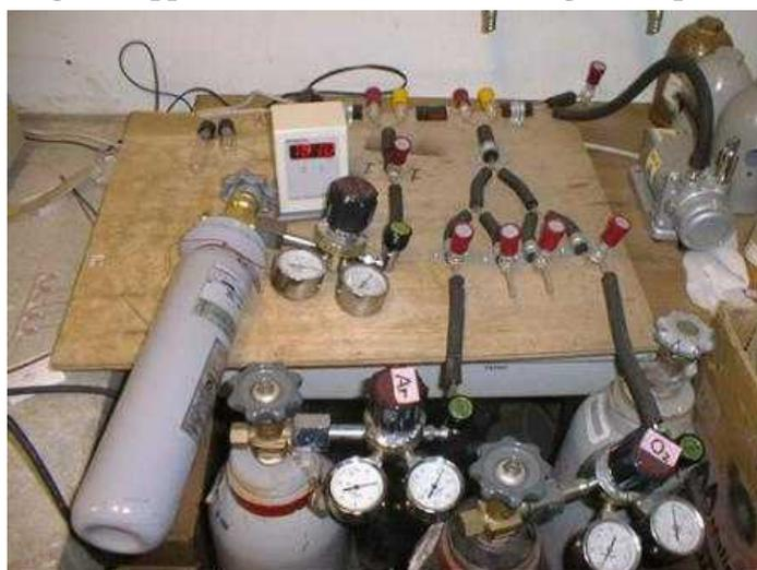
**Fig 11: Gas mixing apparatus for  $^{15}N_2$  fixation studies**
