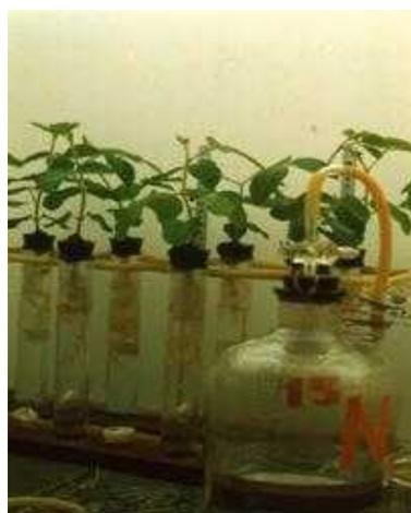
**Fig. 9: Apparatus for  $^{15}N_2$  fixation of intact soybean plants**
