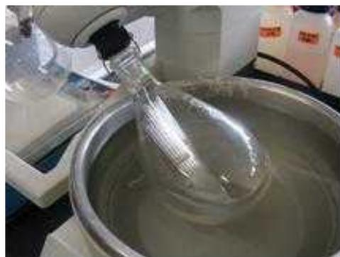
**Fig. 14: Evaporation of water in Kjeldahl digested solution in Pyrex glass tubes by round bottom flask with short neck**
