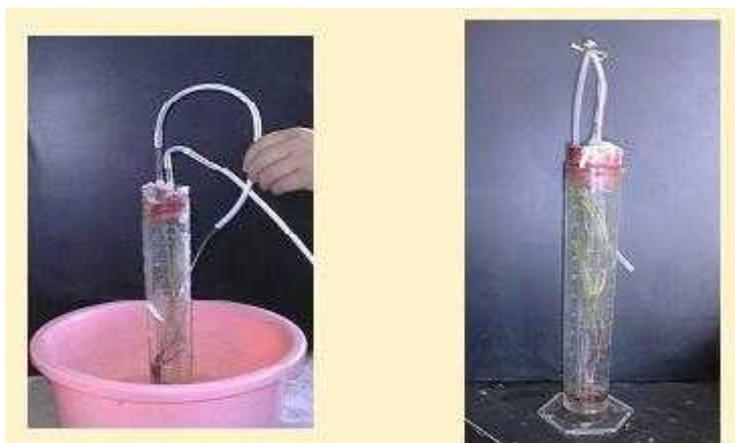
**Fig. 10: Apparatus for  $^{15}N_2$  fixation for sugarcane plants**
