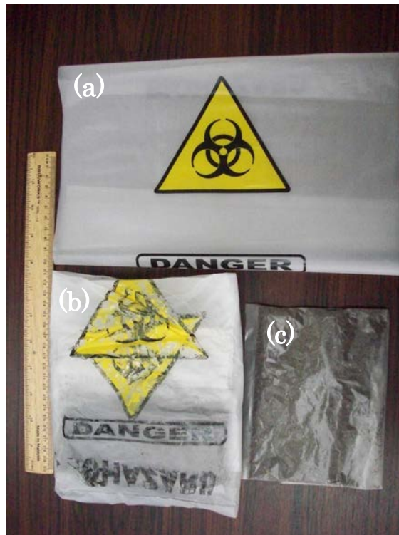
Figure 8: (a) Autoclave bag for packing, (b) carriers sterilized by autoclaving and (c) gamma sterilized carrier
