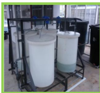
Fertigation system using liquid biofertilizer
