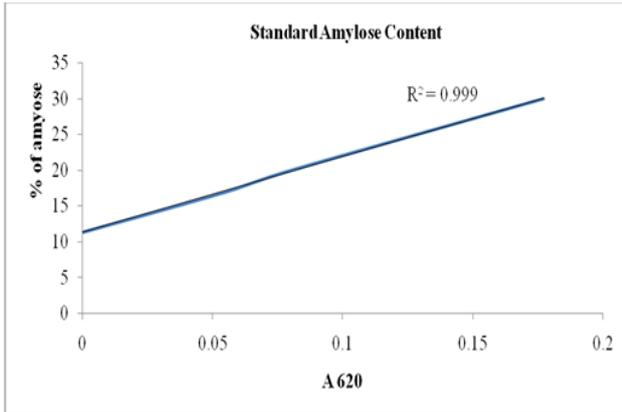
Figure 14. Standard curve of amylose using UV-VIS Spectrophotometer
