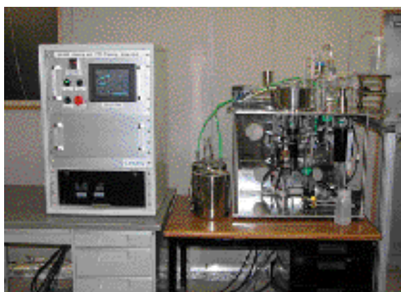
Automatic loading machine for Mo-99 adsorbed PZC
