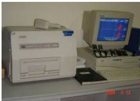
Figure 4: The TLD Reader HARSHAW 4500
