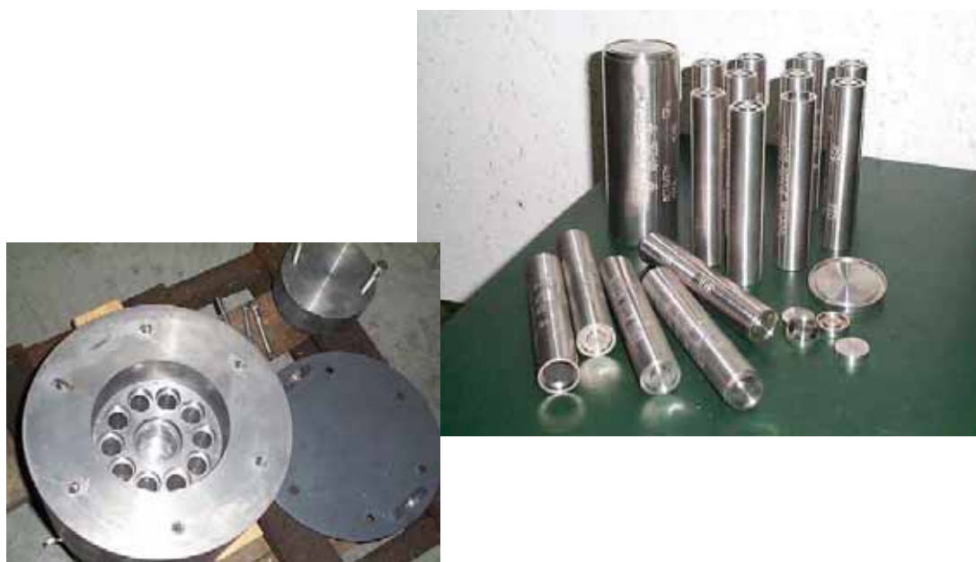
Fig. 2 The small stainless steel capsules and the big sized capsule shown with the steel lined lead container for the ten small capsules and one big capsule
