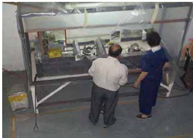
Fig. 1 Working bench/area showing the three distinct zones: the transfer zone, the welding zone and the leak testing zone
