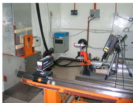
Figure 4: Calibration of survey meter using x-ray machine
