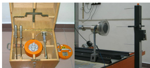
Figure 2: Standardization of ^{90}\text{Sr}/^{90}\text{Y} beta sources (1.85 GBq and 74 MBq) using extrapolation chamber
