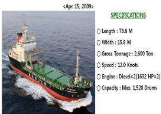
Figure 3: Cheong Jung Nuri (Radioactive Waste Transport Ship)
