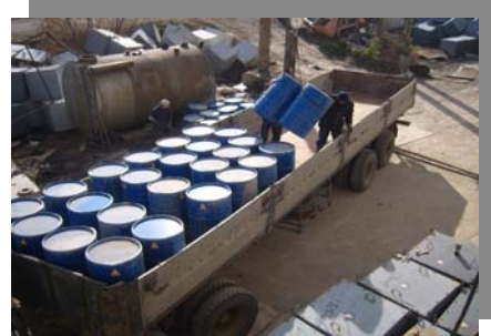
Fig1: The loading of casks with cemented RW into cargo truck
