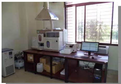
Fig2: Atomic Absorption Spectrometer
