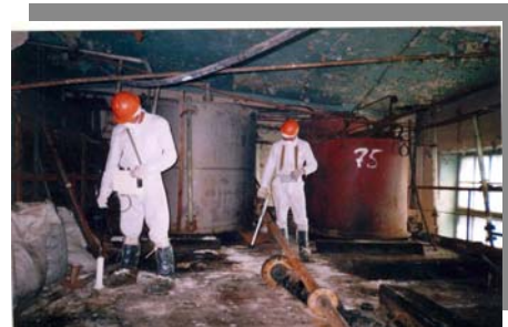
Fig2: Radiation survey in operating workshop
