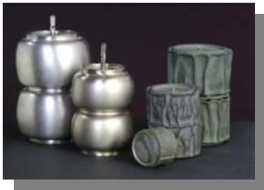
Fig3: Pre- (left) and Post- (right) HIPed cans
