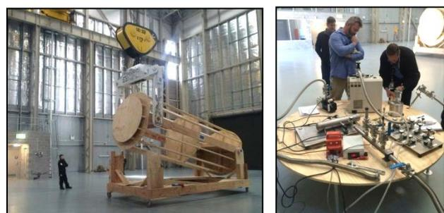
**Figure3:** Hands-on training (a) Use of building crane to lift and tilt a mock-up TN81 cask from the transport frame (b) Test run of leak tightness equipment set up on a mock up secondary lid.
