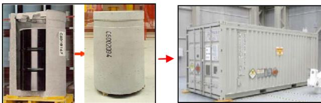
**Figure1:** The cemented technological wastes are cemented within overpacks and placed inside an ISO IP2 transport container, DV78.
