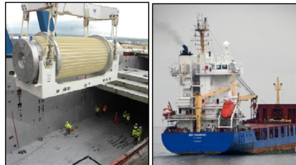
**Figure2:** TN-81 Cask being loaded onto a Class INF2 ship
