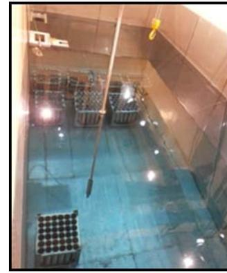
Figure1: Transferring spent fuel from rack to sipping test basket
