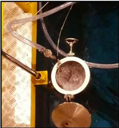
Figure5: Stirring water inside sipping test tube
