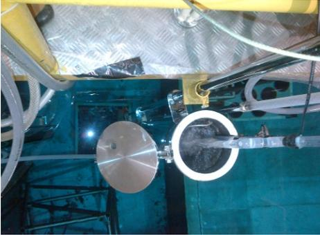
Figure3: Filling sipping test tube with demineralised water
