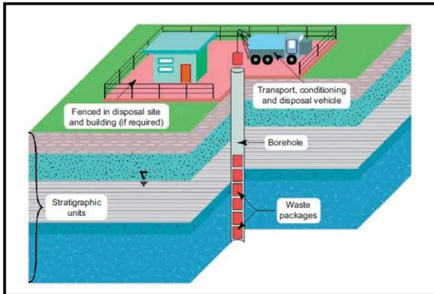
Figure2: Schematic layout of a borehole disposal concept (Ref 1)
