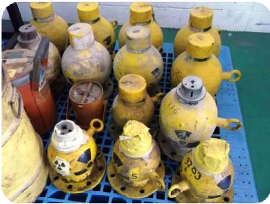
Figure1: Disused sealed radioactive sources
