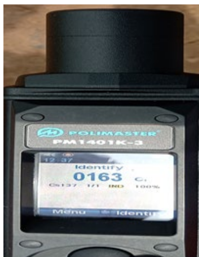
Fig.1. Radionuclide detection in contaminated material using radio isotope identification device
