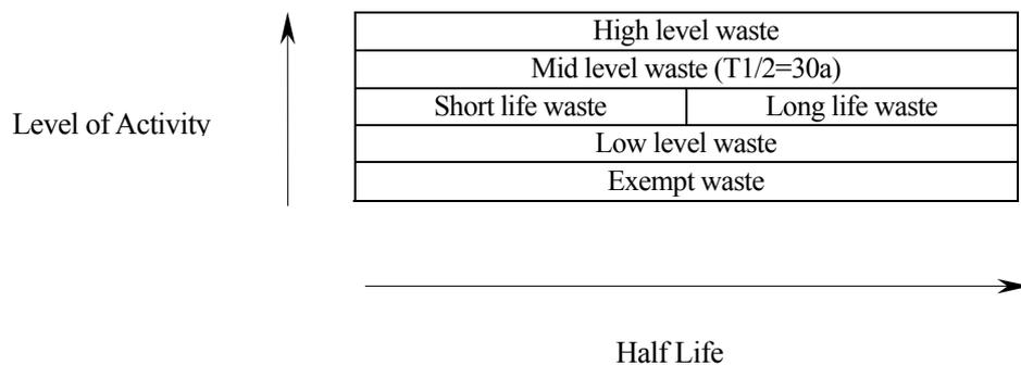
Figure 3.2-3 Framework of Classification for Radioactive Waste
