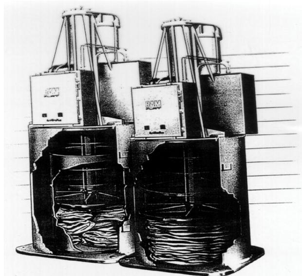
Figure 3.7-7 Drum and In-drum Compactor
