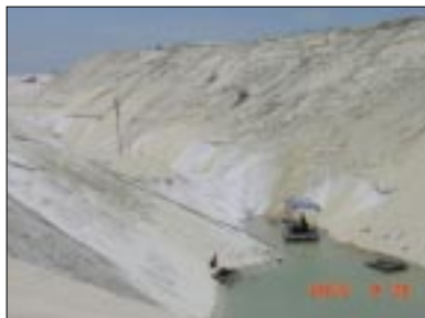
The black beach sand is pumped up with white sand and sea water from the bottom of pond.
