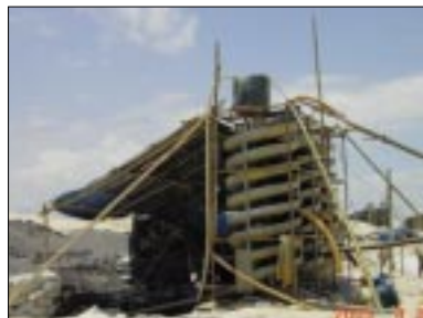
The black beach sand is separated from white sand by the cyclone separation method.
