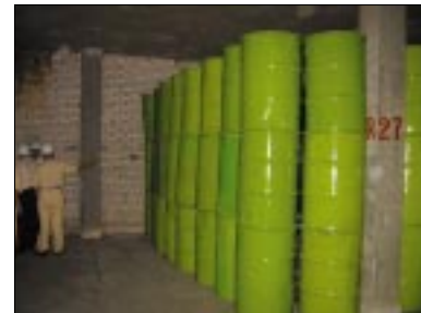
80,000 drums of Th waste has been stored in the LTSF. The maximum dose rate at the surface of drum can be 200µSv/hr.
