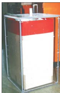
Cardboard box with red bag as the inner liner in a Perspex shield box. Suitable for storage Phosphorus-32 waste (strong beta emitter) in the laboratory
