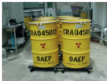
Figure 5 : Ra-226 Conditioned Drums
