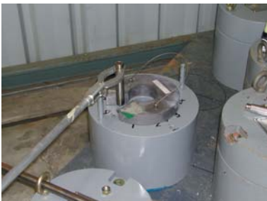
Figure 4 : Placing Ra-226 Capsule
