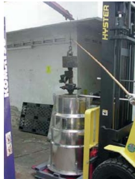
Figure 4 226 Ra (4 Ci) Loading in Pb-Shield
