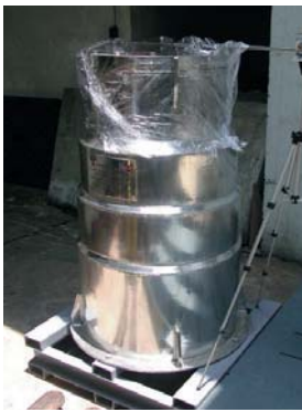
Figure 5 Radon Gas Leakage Test
