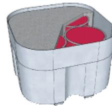
**Conceptual drawing of over pack containers being assessed for use for low level waste conditioning and packaging**
