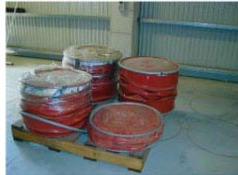
**Super compaction tests conducted using inactive 200 L drums**
