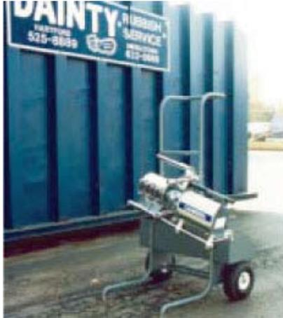
**Commercially available Portable gamma scanner**
