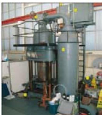
**The 1000 tonne press earmarked for super compacting 200 L drums**
