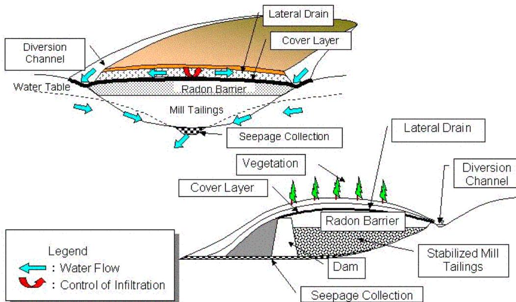
Figure 4.2.3-1 Disposal concept of uranium mill tailings
