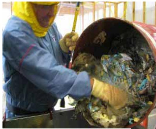
**Fig: 16:** Exempt Level Waste removed from drums for clearance and disposal
